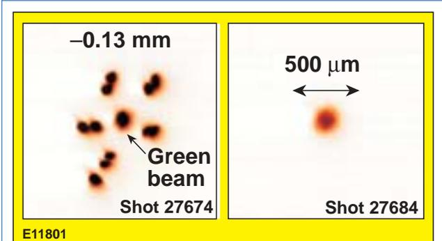
Figure 1. Pointing shot (27674) on a gold sphere. The double spots arise from the distributed polarization rotators (DPR's) on  $3\omega$  beams. There are no phase plates on any of the beams and no DPR in the green probe beam. Shot 27684 shows the green beam only, focused on a pointing target with a DPP producing a 200- $\mu\text{m}$  spot.
