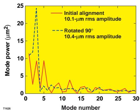
Figure 2. Measured  $\text{D}_2$  ice layer nonuniformity for a CH shell of  $\sim 920\text{-}\mu\text{m}$  diameter and 3.5- $\mu\text{m}$  wall containing a 100- $\mu\text{m}$   $\text{D}_2$ -ice layer. The solid line is the measurement from the initial target alignment, and the dashed line is the measurement for the target rotated by  $90^\circ$  from the original orientation.
