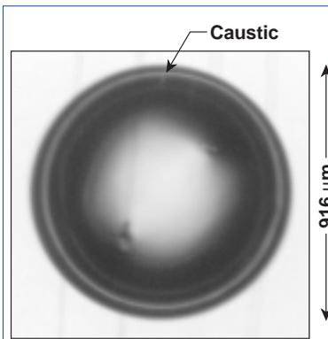
Figure 1. Shadowgram of 3.6- $\mu\text{m}$ -thick, 916- $\mu\text{m}$ -diam CD shell containing an 80- $\mu\text{m}$ -thick  $\text{D}_2$ -ice layer. The bright band is a caustic generated by the ice/gas interface. Detailed analysis of this band produces a measure of the uniformity of the ice layer. This measurement can be carried out with a spatial resolution of 1 to 2  $\mu\text{m}$ .
