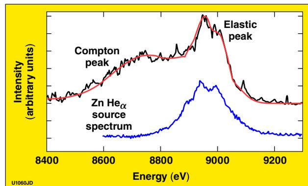
Figure 2. In-flight x-ray scattering spectrum from laser-compressed CH cone-in-shell targets, including an elastic feature and a Compton downshifted peak. Theoretical fits to the experimental data yield temperature, densities, and ionization states of about  $0.8 \times 10^{24} \text{ cm}^{-3}$ , 11 eV, and C(+3)H(+1). Also plotted is the Zn He $\alpha$  probe source spectrum (blue).
