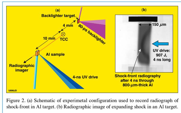
Figure 2. (a) Schematic of experimental configuration used to record radiograph of shock-front in Al target. (b) Radiographic image of expanding shock in an Al target.
