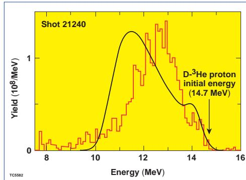
Figure 1. Measured (red) and simulated (black) proton spectra for a 20-μm-thick, 969-μm-diameter CH shell filled with 15 atm D<sup>3</sup>He and irradiated with 22.8 kJ of UV energy. The 1-D calculation has been scaled by the ratio of the experimental to 1-D proton yields.
