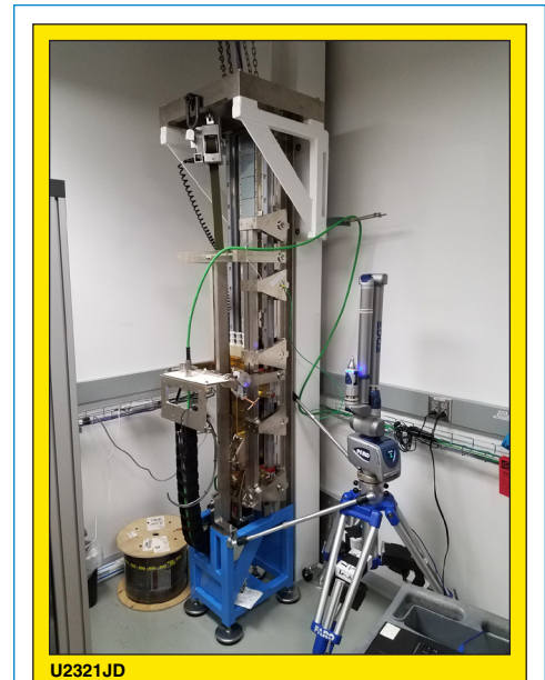
Figure 1. The new linear motor is shown mounted in the lab test fixture (blue and white components). A 3-D coordinate measuring machine (tripod, lower right) was used to verify alignment accuracy during assembly.
