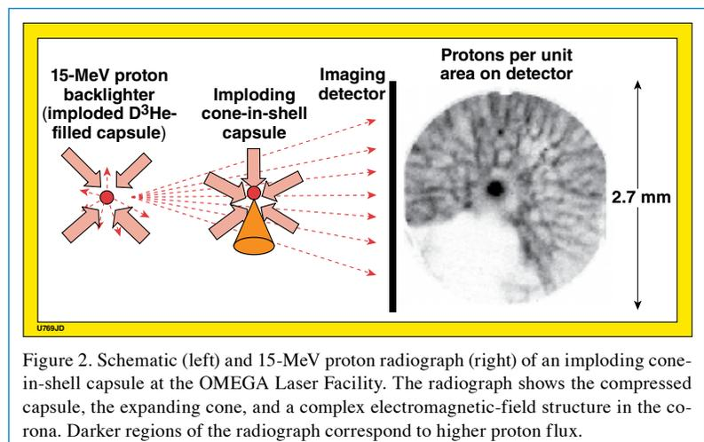
Figure 2. Schematic (left) and 15-MeV proton radiograph (right) of an imploding cone-in-shell capsule at the OMEGA Laser Facility. The radiograph shows the compressed capsule, the expanding cone, and a complex electromagnetic-field structure in the corona. Darker regions of the radiograph correspond to higher proton flux.
