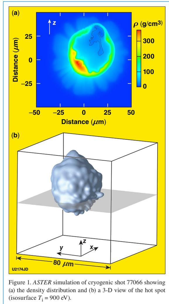
Figure 1. *ASTER* simulation of cryogenic shot 77066 showing (a) the density distribution and (b) a 3-D view of the hot spot (isosurface  $T_i = 900 \text{ eV}$ ).
