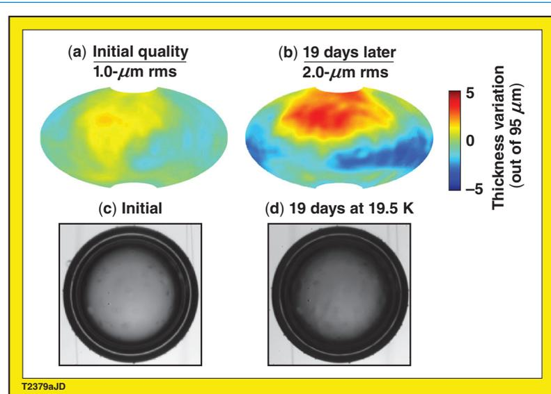
Figure 2. The increase in roughness of an ice layer that was allowed to age for 19 days is shown using Aitoff projection [Figs. 2(a) and 2(b)] and shadowgrams [Figs. 2(c) and 2(d)]. The latter images show no evidence of  $^3\text{He}$  bubbles forming within the ice.
