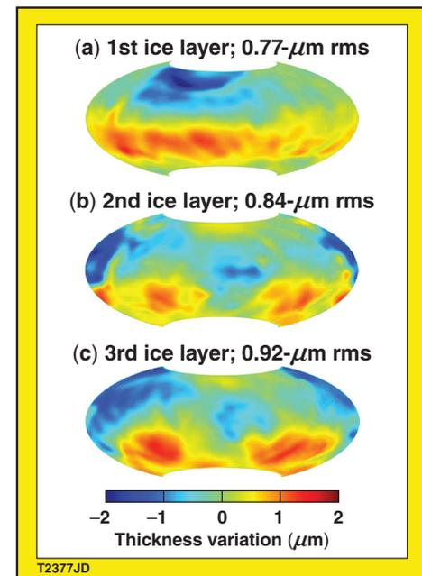
Figure 1. The variation in the thickness of a  $95\text{-}\mu\text{m}$  ice layer is shown using Aitoff projection of the analyzed shadowgrams. Three separate ice layers, formed in the same plastic capsule [(a)–(c)] demonstrate the repeatability of the process: the rms roughness of each layer is comparable.
