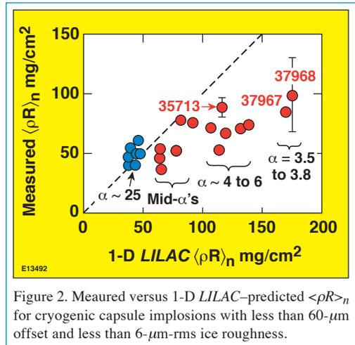
Figure 2. Measured versus 1-D *LILAC*-predicted  $\langle \rho R \rangle_n$  for cryogenic capsule implosions with less than 60- $\mu$ m offset and less than 6- $\mu$ m-rms ice roughness.
