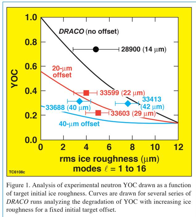
Figure 1. Analysis of experimental neutron YOC drawn as a function of target initial ice roughness. Curves are drawn for several series of *DRACO* runs analyzing the degradation of YOC with increasing ice roughness for a fixed initial target offset.
