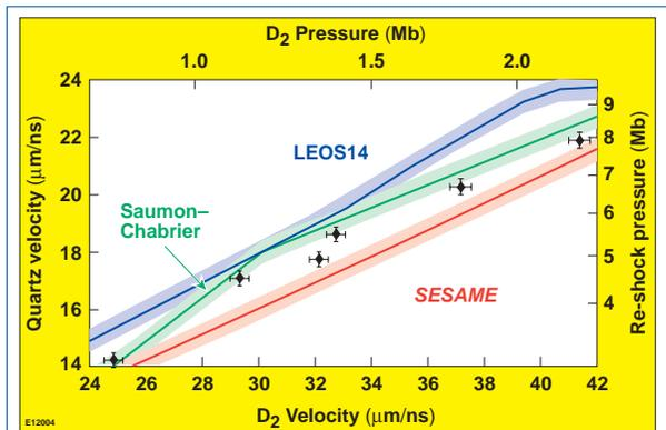
Figure 2. Plot of quartz shock velocity (re-shocked  $D_2$  pressure) versus  $D_2$  velocity ( $D_2$  pressure) measured in the experiment. For comparison, note the *SESAME*<sup>1</sup> table predictions (solid red line), LEOS14 (a fit to the NOVA data<sup>3</sup>), and the Saumon–Chabrier model.<sup>2</sup> The measurements use quartz as a reference material; the bands represent anticipated excursions due to worst-case uncertainty in that reference.
