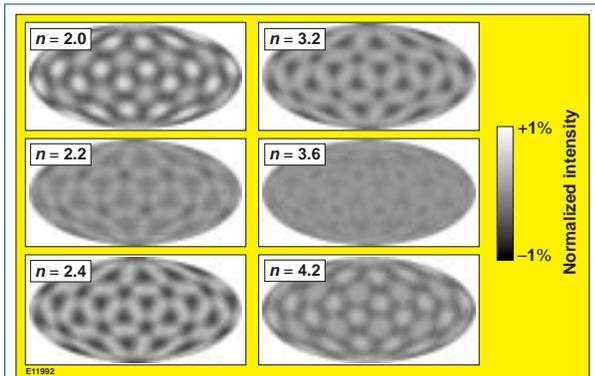
Figure 1. Aitoff projections of the spatial variation of absorbed energy on OMEGA spherical targets with DPP's producing a super-Gaussian intensity distribution of varying order,  $n$ . These calculations assume that the absorption varies as the cosine of the angle to the target normal.
