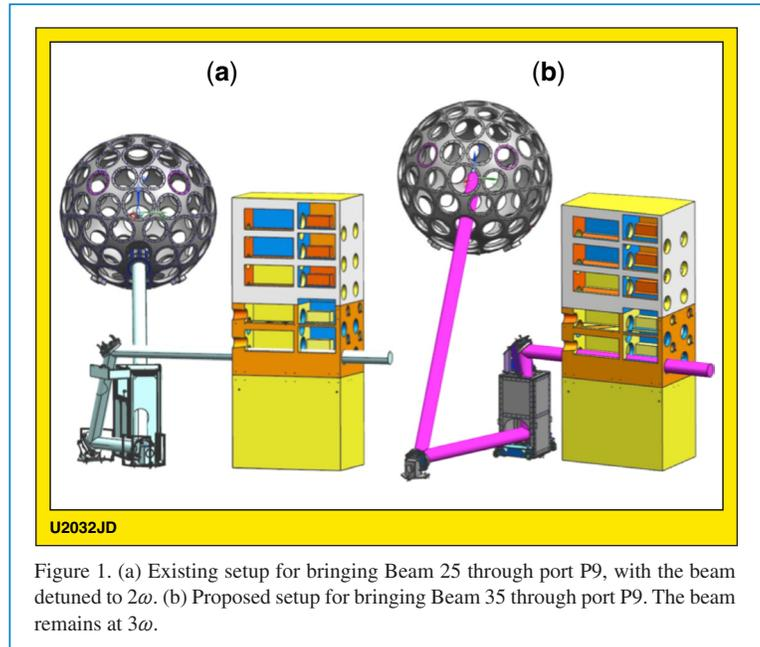
Figure 1. (a) Existing setup for bringing Beam 25 through port P9, with the beam detuned to  $2\omega$ . (b) Proposed setup for bringing Beam 35 through port P9. The beam remains at  $3\omega$ .
