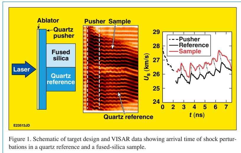
Figure 1. Schematic of target design and VISAR data showing arrival time of shock perturbations in a quartz reference and a fused-silica sample.
