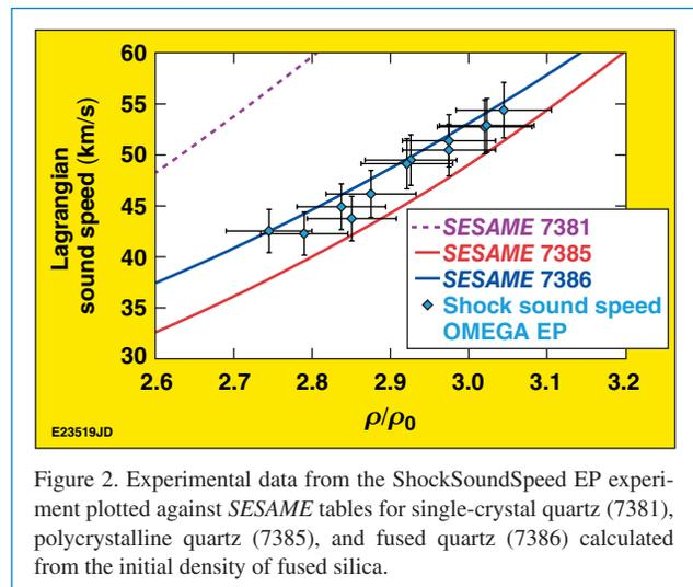
Figure 2. Experimental data from the ShockSoundSpeed EP experiment plotted against *SESAME* tables for single-crystal quartz (7381), polycrystalline quartz (7385), and fused quartz (7386) calculated from the initial density of fused silica.
