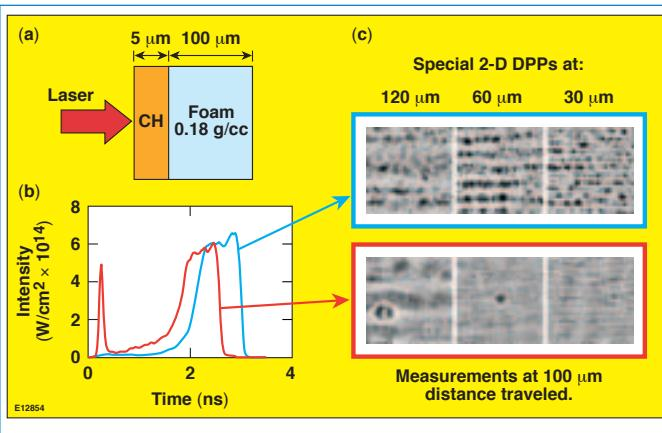
Figure 1. (a) Schematic of the target consisting of a 5- $\mu\text{m}$ -thick plastic foil followed by a 100- $\mu\text{m}$ -thick foam foil with density of 180 mg/cc. (b) On-target laser intensity as a function of time for two pulse shapes with and without picket. (c) Optical-depth radiographs of the targets driven without picket (upper three images) and with picket (lower three images) with 2-D imprinted features at 120-, 60-, and 30- $\mu\text{m}$  wavelengths.
