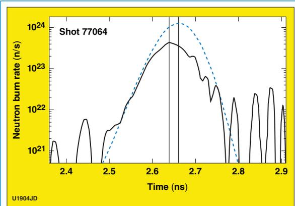
Figure 1. A comparison between the neutron burn rate measured with the P11 NTD diagnostic (solid black line) and the 1-D simulation (dashed blue line). The P11 NTD instrument response function has been applied to the 1-D simulated neutron burn rate.
