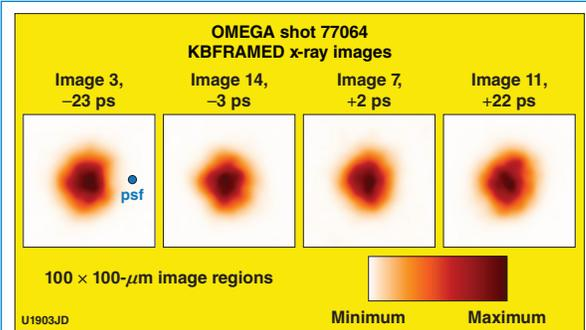
Figure 2. Gated x-ray images of a DT cryogenic implosion in the 4- to 8-keV photon energy range measured with the 16-channel Kirkpatrick–Baez microscope recorded at stagnation for shot 77064. The point spread function (psf) is indicated by the blue circle ( $\sim 6 \mu\text{m}$ ).
