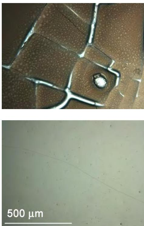
**Figure 40:** Microscope images of cast blend films of 50/50 PS-4/M-PMMA-6 (top) and 50/50 PS-2/M-PMMA-6 (bottom) showing examples of demixed and mixed states, respectively. The scale bar is the same for both images.
