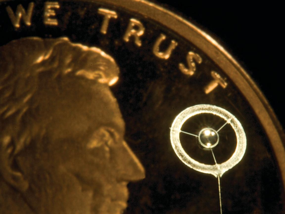
SATURN PDD TARGET Polar direct drive (PDD) has been developed by LLE as a potential means to achieve direct-drive ignition on the NIF in its initial indirect-drive (two-sided) irradiation configuration. The "Saturn" target shown above is a variation of the PDD approach that relies on a plastic ring surrounding the full capsule. Upon laser irradiation, the ring forms a low-density plasma that refracts laser light toward the capsule to optimize the drive uniformity for PDD targets.
