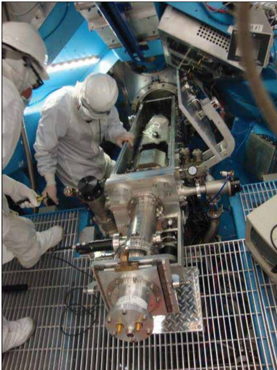
Figure 132.160 Photo of the EHRXI in TIM-1; the CID camera holder sits at the back of the TIM.
