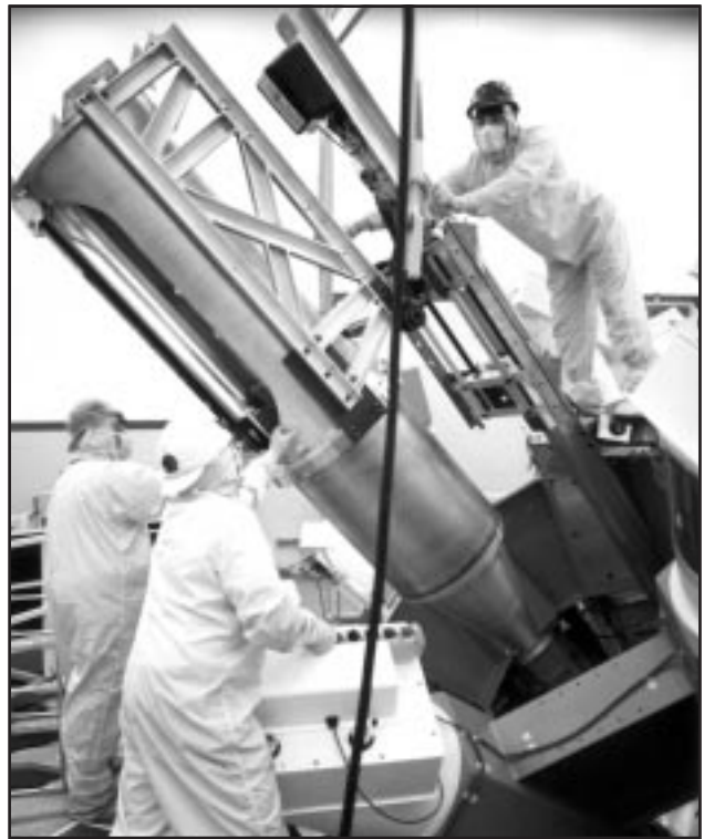
Figure 76.48 Photograph taken during the installation of the second of two charged-particle spectrometers on OMEGA.
