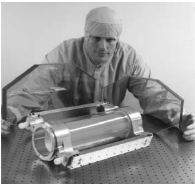
Fig. 3.4-2 UR/LLE-developed LHG-8 laser glass is used in two basic shapes and several sizes. Shown are the hexagonal elements for the 15- and 20-cm disk amplifiers and a 90-mm rod (inside the module assembly).
