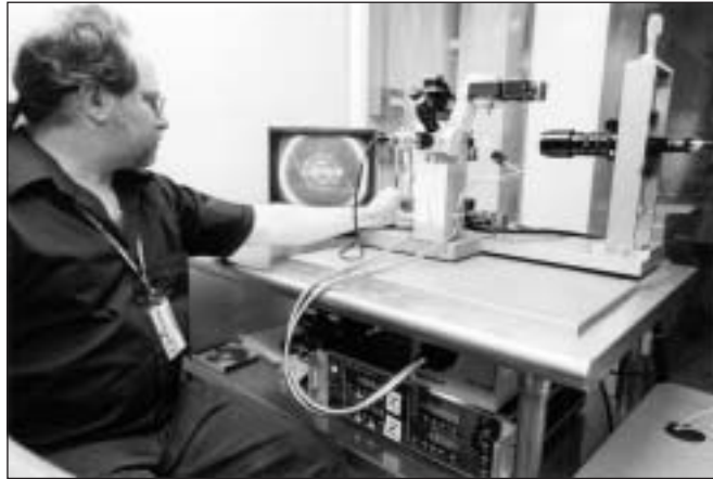
Figure 2.5-1 The Powell scope metrology station. This provides 4° of motion to manipulate the target's position and orthogonal camera views to measure dimensions.
