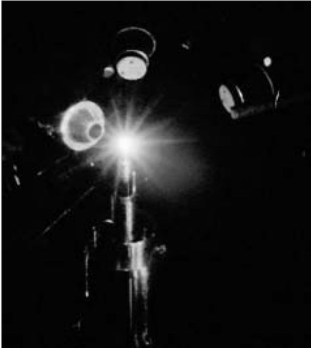
Figure 2.4-6 A photograph of a cryogenic planar shot inside the OMEGA chamber.
