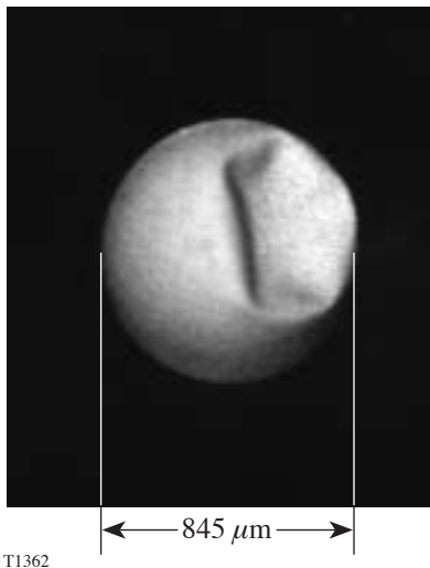
Figure 2.2-7 Target buckled due to external overpressure of 5 atm.
