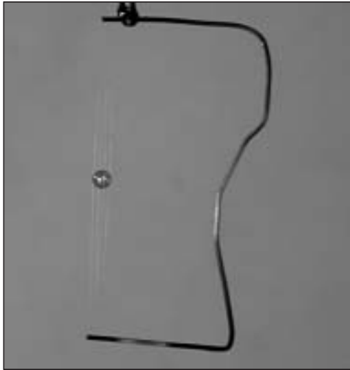
Figure 2.3-1 Spherical target mounted on a convoluted Be frame with four spider silks.
