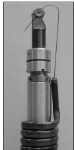
Figure 2.4-5 Fully assembled cryogenic planar target.
