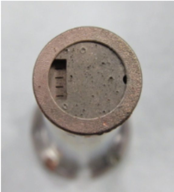
Damage to VSG snout From previous experiment in TIM 14
