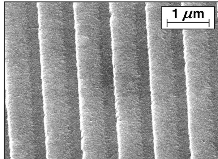
**SEM image of blazed holographic diffraction grating, 1201.6 grooves/mm, blazed for 250 nm**
