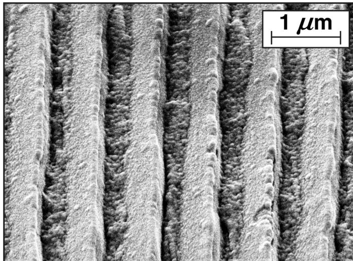
**Scanning electron microscope (SEM) image of mechanically ruled, blazed diffraction grating, 1200 grooves/mm, 36.8° blaze angle**
