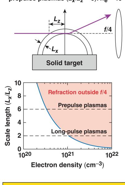
An f/4 system will provide access to highly refractive plasmas.
