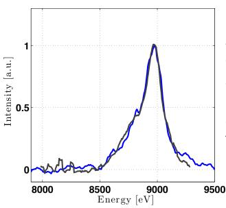
Scattered spectrum collected with the zinc spectrometer. Analysis indicates a weighted average electron temperature of ~35 eV.
