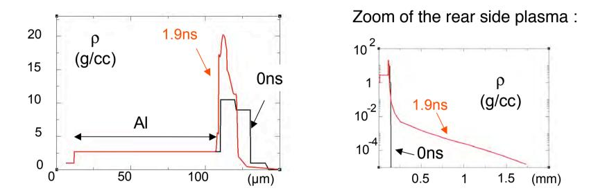
The LP beam creates a several 100s  $\mu$ m-long coronal plasma at the target's rear side
