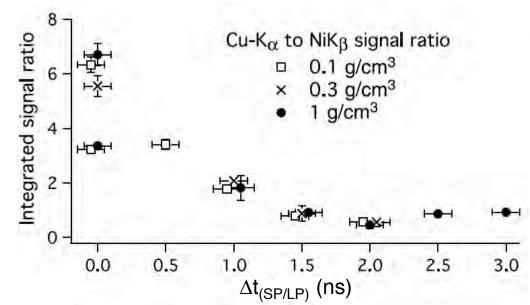
The fraction of electrons reaching the target rear surface decreases during compression ∀ρ₀ (no clear dependence on the initial foam density)
