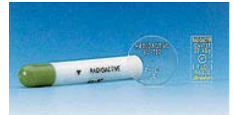
Radio active sources: Am-242, Cd-109, Co-57
