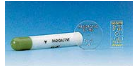
Radio active sources: Am-242, Cd-109, Co-57
