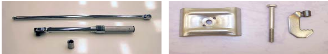
Figure 1: (a) Required tools; (b) Grating tie-down assembly
